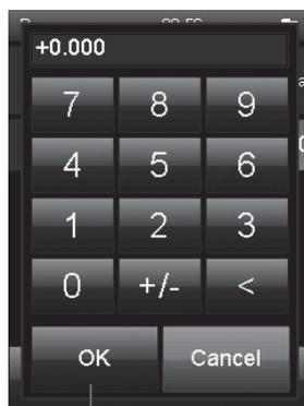
Using the keypad in fig. I, enter the deviation of the current measured value (3) from the reference value.
