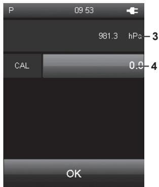
For air pressure measurement a 1-point adjustment is available
