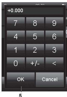
Using the keypad in fig. J, enter the deviation of the current measured value (3) from the reference value.
