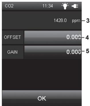
For CO<sub>2</sub> probes an offset / gain adjustment is possible.
