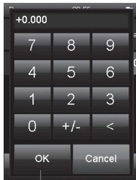
Using the keypad in fig. H, enter the deviation of the current measured value (3) from the reference value.
