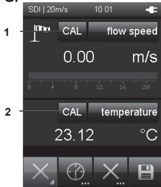
In measurement mode press button CAL (1) or (2) in order to switch to customer adjustment mode (fig. G).
