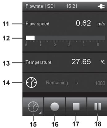
11 Shows the measured flow rate as a numerical value in the selected unit (e.g. m/s).
