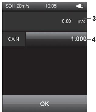
Select the value field (4) in either fig. H or fig. I to adjust the current measured value (3).
