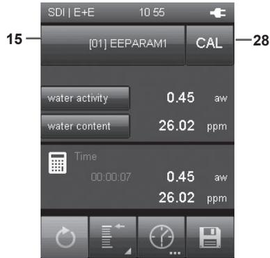
The measurand "water content [ppm]" is a calculated value. For this calculation oil specific parameters (A und B) are needed. The default factory parameter set is [01] EEPARAM1, which contains oil specific parameters for mineral transformer oil. The determination of other oil-specific parameters can be performed by E+E on request.
