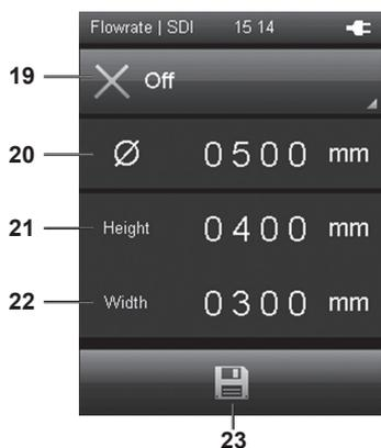
19 Selects the form of the object to be measured. The following options are available (see fig. F.)::
